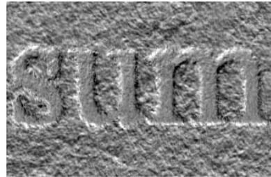
Figure 3. Difference image between two 1200 DPI scans showing the surface texture measured by the scanner in the y direction. Actual size: “sum”.
